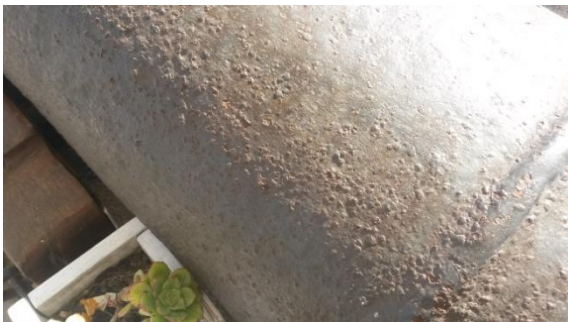
The 8pdr with corrosion blisters in April 2015, before the restoration.
